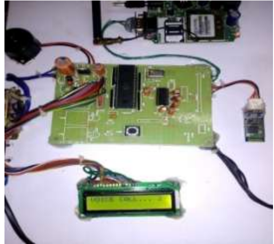
Fig The gsm module makes a voice call to the 2 st number.
