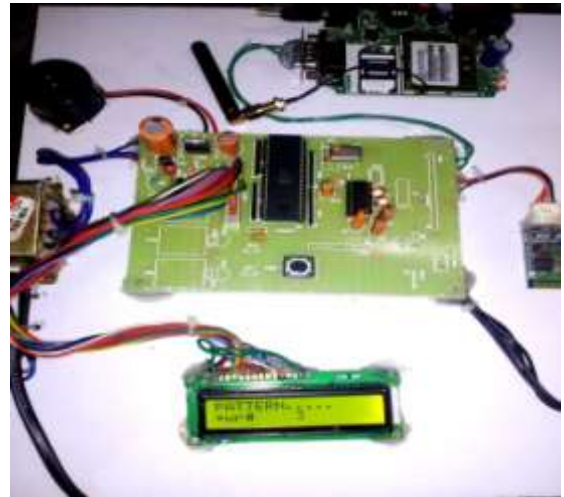
Fig If an intruder enters a wrong pattern for the first time it will display *wr# 3 in the LCD.
