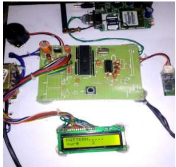
Fig If an intruder enters a wrong pattern for the second time it will display *wr# 2 in the LCD.
