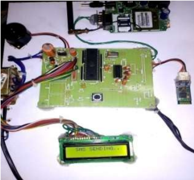
Fig If an intruder enters a wrong pattern for the third time then the buzzer will ring to alert the neighbours and a sms alert will be sent to the 3 numbers along with a voice call which are in the microcontroller.
