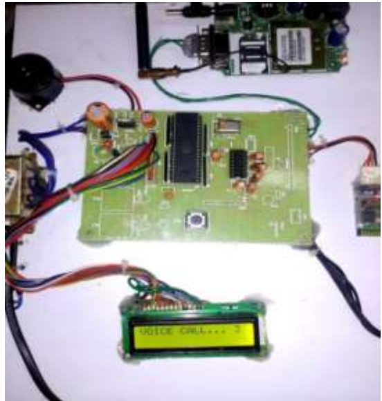
Fig The gsm module makes a voice call to the 3 rd number.
