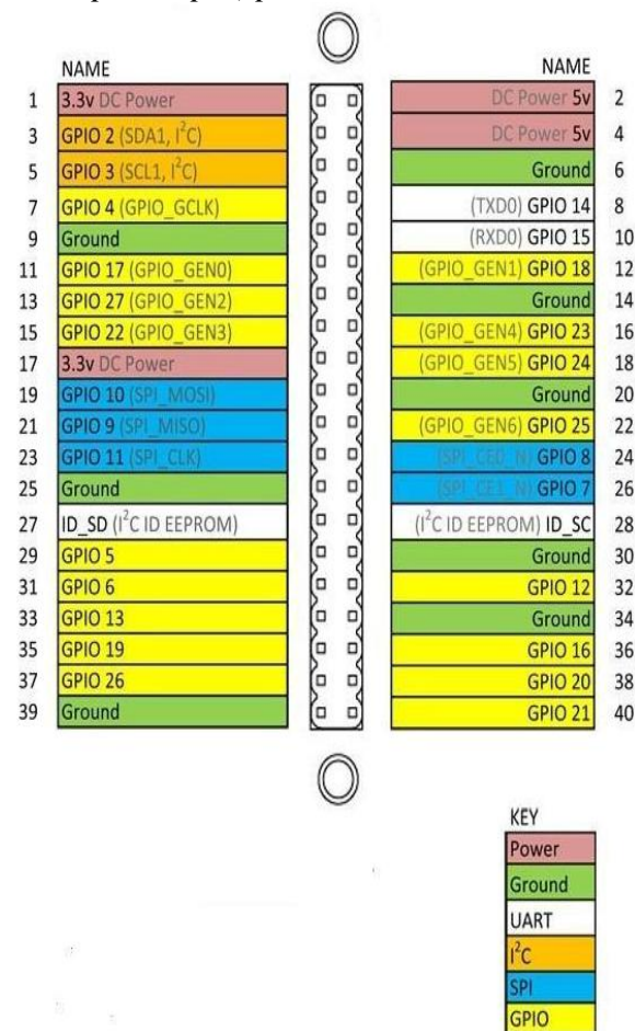
Figure 2: GPIO Pin Configuration
