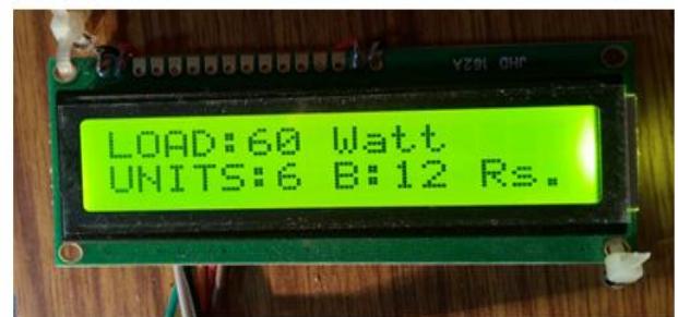
Figure 6: Hardware of Smart Energy Meter The above fig.6 illustrates the overview of the IOT based smart energy meter reading using Raspberry Pi3. Here we use raspberry pi3, Energy Meter, LCD display and optocoupler. The billing of the electricity consumed is implemented through Raspberry Pi3.
