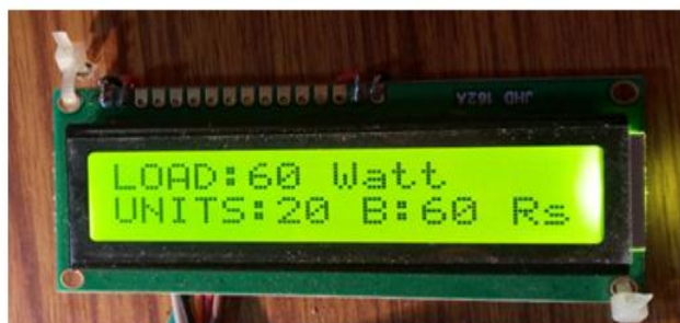
Figure 7: LCD Display of Energy Billing and Consumed Units
